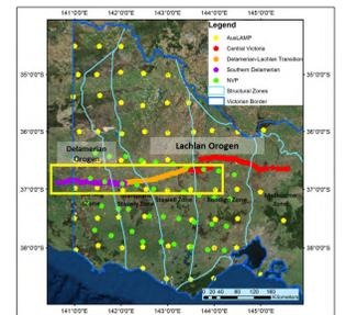
Figure 1: Location of the MT sites in Victoria. Yellow sites are part of the Australia-wide AusLAMP project involving collection of long-period (deep sounding) MT data every 0.5 degrees. All sites shown are used in Figure 3, and only the sites in the yellow box are used in the inversion shown in Figure 5.
