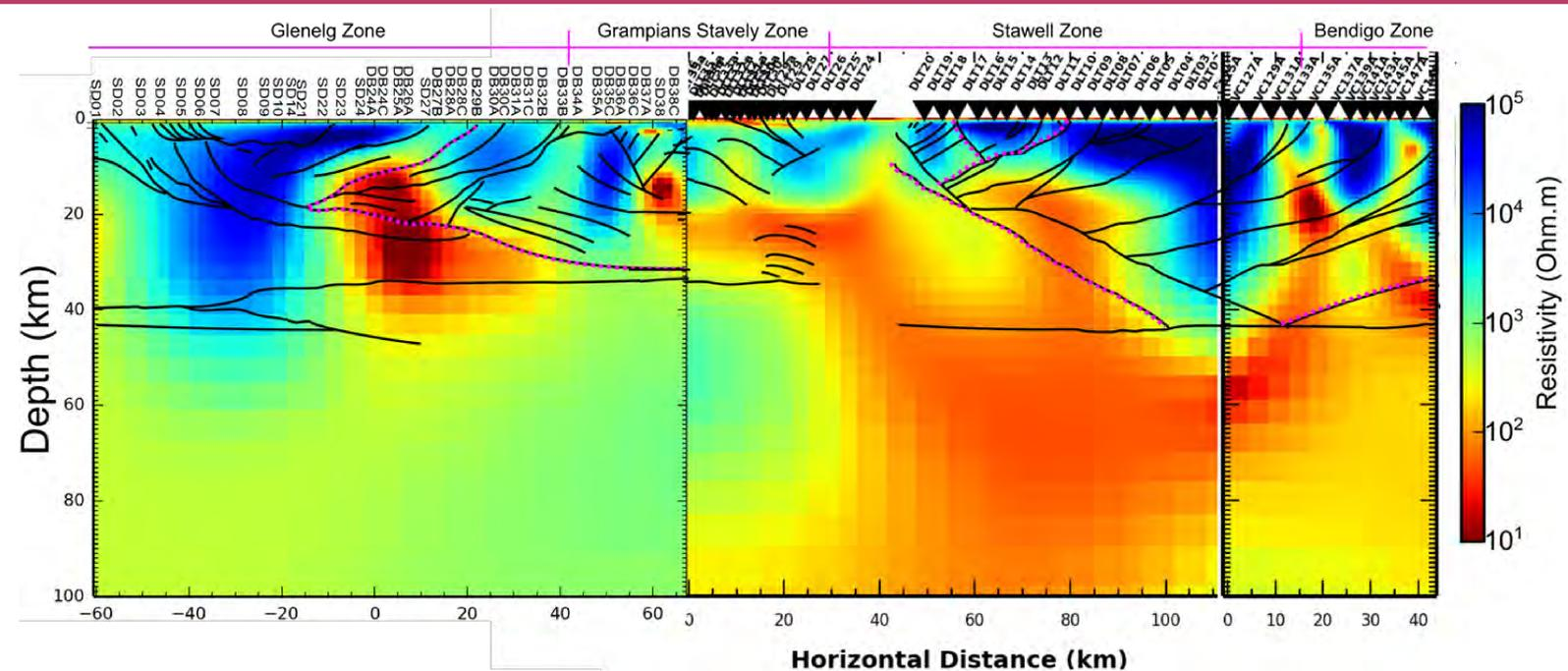
Figure 5: Electrical resistivity slice from the surface to 100 km depth, along the profile of sites in the yellow box from Figure 1. Black lines are faults interpreted from deep reflection seismic surveys (Cayley et al., 2011). Red indicates conductive regions, blue are resistive.
